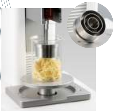
TX-TRPF : THREE RINGS PROBE CUTTING FIXTURE (Ref. 130186)
