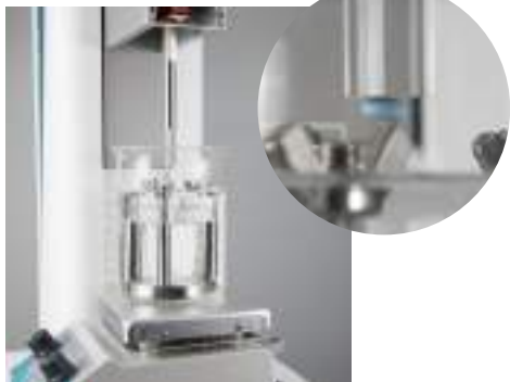
TX-MAF : MUCO ADHESION FIXTURE (Ref. 130181)
