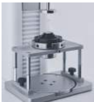
TX-SAF : SYRINGE ACTUATOR FIXTURE (Ref. 130145)
