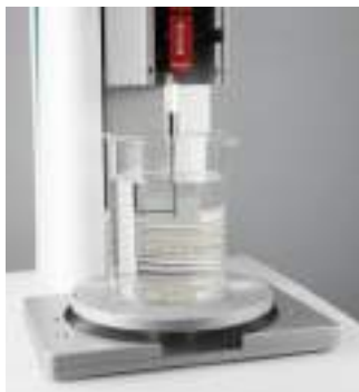
TX-RSF : RAFT STRENGTH FIXTURE (Ref. 130021)
