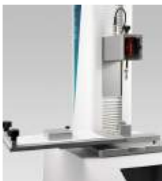
TX-SFF : SLIDING FRICTION FIXTURE (Ref. 120013R)
