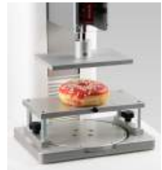
TX-CTPF : COMPRESSION TOP PLATE FIXTURE (Ref. 130153)
