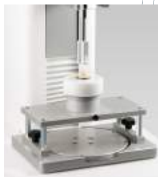
TX-DSF : DOUGH STICKINESS FIXTURE (Ref. 121017)
