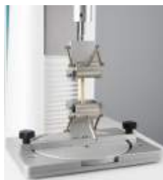
TX-RTF : ROLLER TENSILE FIXTURE (Ref. 130194)
