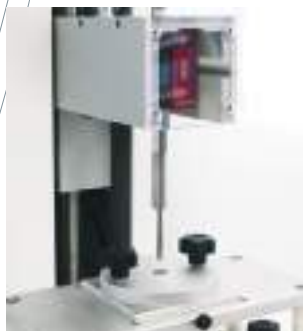
TX-FCF : FILM COMPRESSION FIXTURE (Ref. 130031R)
