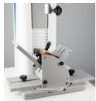
TX-GPJF : GENERAL PEELING JIG FIXTURE (Ref. 310105R)
