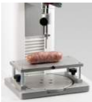
TX-MP : MOHRS PROBE (Ref. 130165R)
