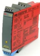
Isolator Used with AMT-Ex & DS4000 in the Safe area
