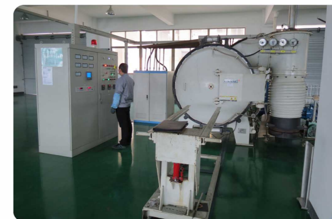
Vacuum brazing furnace
