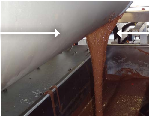
2. Mixing unit on top of the molds for adding: - Nuts, salt, other particles - Liquid additives
