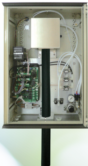
internal view with heated line connection
